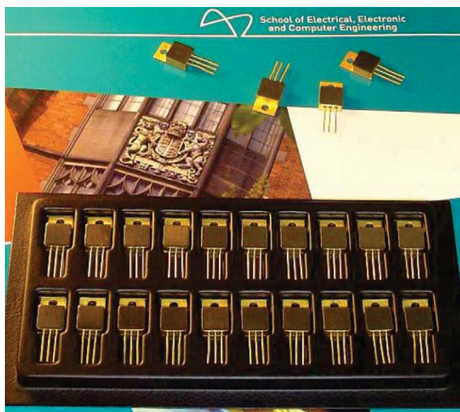
Fig. 3 Packaged SiC Schottky diodes.
